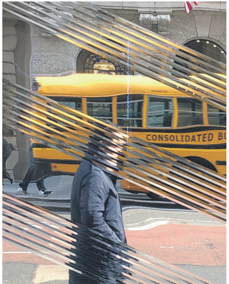
Groove grinding: Rippled glass can be used as a privacy screen or as a pure design element. The grooves in the glass refract the light and create a charming play of light.
